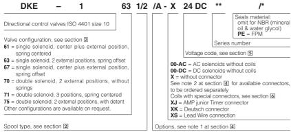
Spool type, direct operated valves with threaded solenoids certified according the North American standard **cURus**
