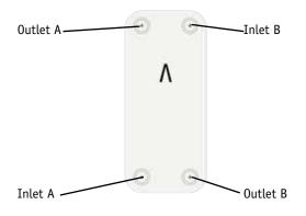
Maximum cooling efficiency is achieved by cross flowing through the plates, the oil inlet and water inlet being located on a diagonal. Failure to have the cooler attached in this manner will lead to a decrease in efficiency.
