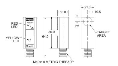
ALS Switch output states may be influenced by an external magnetic field. Care must be taken to avoid external magnetic field exposure.
