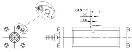
Note: Specify piston code '7' in cylinder model number when using ALS Switches.
