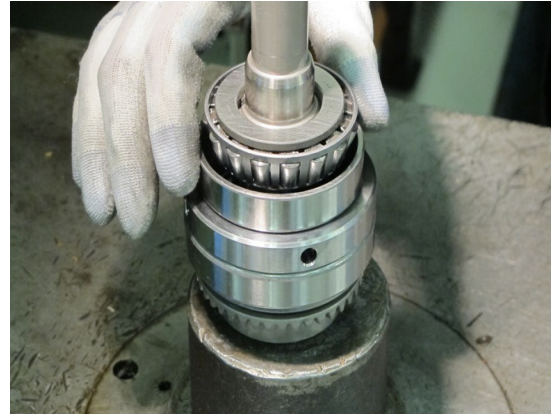
4. Place the small tapered roller bearing on the shaft as on the picture.
