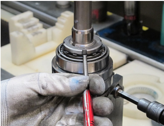
8. Secure the round nut as shown in the picture.
