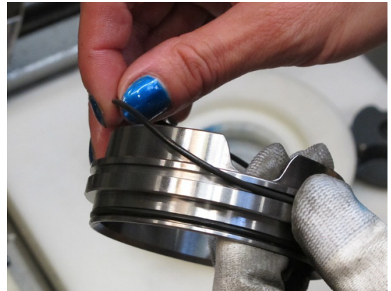
11. Assemble the O-rings on the distance ring.
