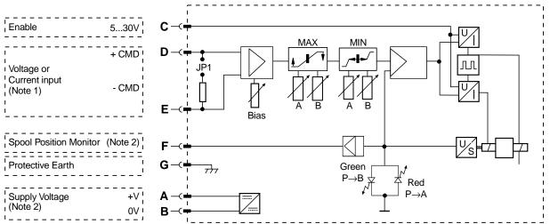
Note 1: Install jumper JP1 for current command input. Refer to Installation Bulletin 2583-M1/USA (D1FX). Note 2: Refer to specifications.
