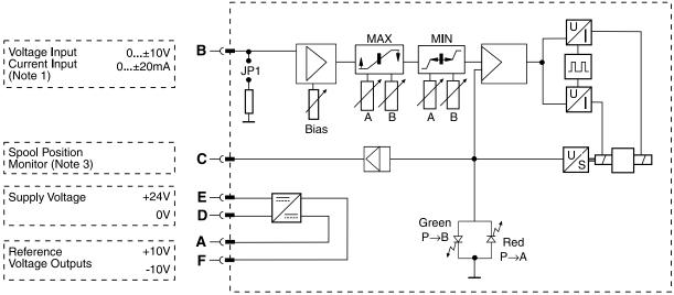
Note 1: Install jumper JP1 for current command input. Refer to Installation Bulletin 2583-M1/USA (D1FX). Note 2: Refer to specifications.
