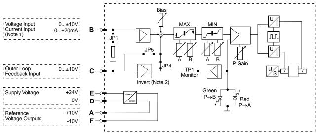
Note 1: Install jumper JP1 for current command input. Refer to Installation Bulletin 2583-M1/USA (D1FX).
