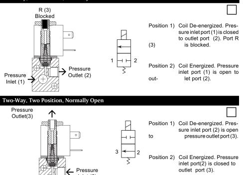
\*Port (1) is permanently blocked. (Both Ends)
