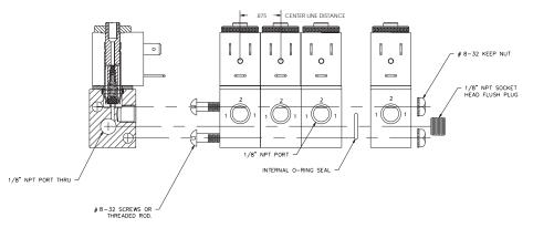
The pressure inlets are located on either end of the manifold assembly with the cylinder port (2) located on the lower block face. On 3-2 way versions the exhaust port R (3) is located on the stem of the valve.
