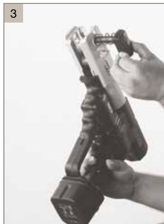
Open the retaining pin at the front of the machine by pressing the jaw release button
