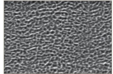
Parker's Global Shield coating features a sub-micron structure (shown here magnified 4000 times) that eliminates surface micro-cracks and delamination.
