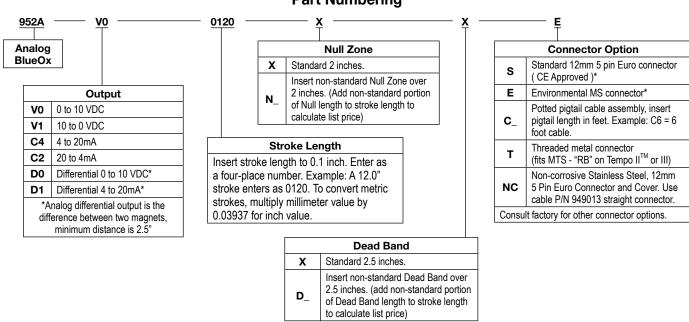
**Note 1:** On unsupported stroke lengths greater than 4 feet, rod support bracket(s) and a special magnet should be used. **Note 2:** Specify magnet as separate line item (standard magnet is SD0400800).
