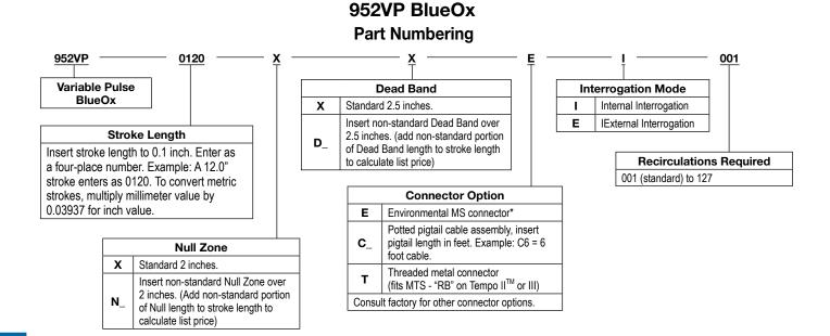
\* If option E (environmental connector) is selected, mating connector and/or cable assembly must be ordered separately.
