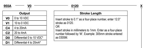
\*Analog differential output is the difference between two magnets. Minimum distance is 2.5".
