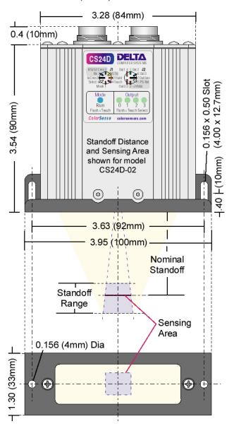
The CS24D is available in several models with a variety of sensing areas and standoff ranges. Standoff ranges include 0.63 to 1.00" (16 to 25mm) and 1.50 to 2.13" (38 to 54mm) shown above.
