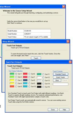
To Teach the CS24D to another object, select another Sort Output and press the Teach button to take the 8 readings. Click the **Done** button when the sensor has been trained to all of the samples.
