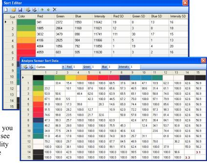
CAUTION: In order for the standard deviation prediction to be correct, it is essential that the Teaching be done optimally. All eight Teach readings must be taken, the eight readings must include representative samples of the range of colors that are considered permissible for that Sort Output, and the sample objects
