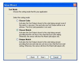
**Closest Match** not only finds the closest match between the Teach colors and the current color, but also requires that the calculated error on the match be less than the **Error Limit** (more later). Otherwise the sensor reports a "no match" condition with all outputs OFF. **Closest Match** mode provides more intuitive operation for the majority of applications.
