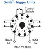
Wiring for 11-Pin Control
