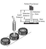
If the hole is present in the gear, the sensor will shine through the hole and ignore the belt—no detection event will occur.
