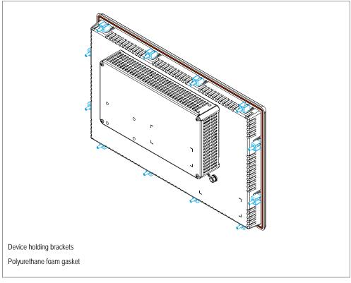
Abb. 3 Fixing and sealing
