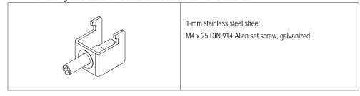
Abb. 5 Device holding bracket
