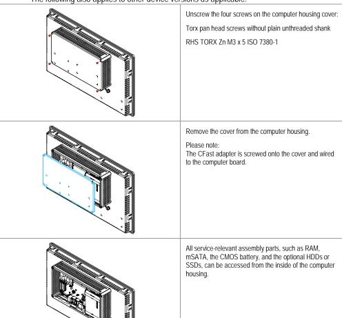
Abb. 7 Opening the device
