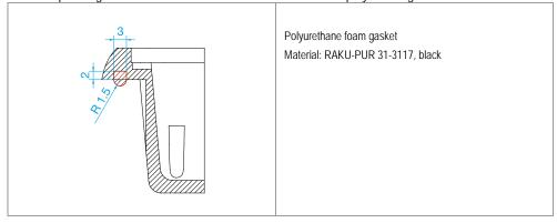
Abb. 4 Polyurethane foam gasket
