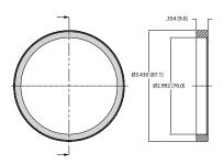
Magnetic Ring (press fit) for pulse rate: 1600, 5120, 6400, 16000
