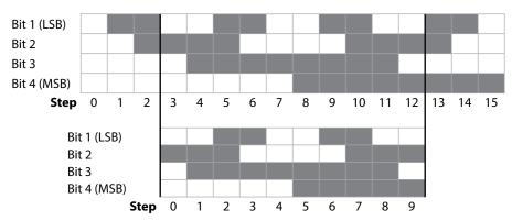
**Reversion of the gray code:** The code values increase when the shaft is turning clockwise. If the most significant bit (MSB) is inverted, the code values decrease when the shaft is turning clockwise.
