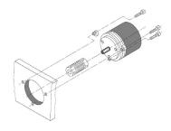
Mounting with assembly bell, fastening eccentrics and coupling (to prevent shaft overload and to insulate the encoder thermally and electrically).
