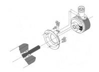
Mounting Examples for Shaft Encoders with Servo Bracket:
