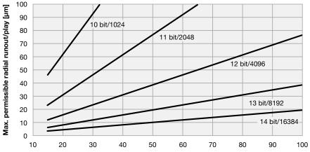
Distance between torque stop locating point and mid-point of drive axle [mm]
