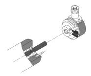
Mounting of a hollow shaft encoder with a flex coupling.
