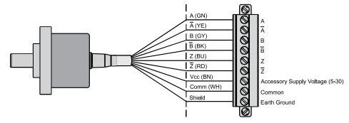
For general industrial environments where there are no large motor or drives present, the standard M12 Eurofast® cordset with non-twisted pair conductors will suffice. In heavy industrial environments, or when used on AC vector motors, M12 Eurofast cordsets with twisted pairs should be used.
