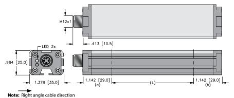
**Ordering Information**The Q-track linear position sensors are available in different lengths from 100 to 1,000 mm, in increments of 100 mm. The sensors, mounting accessories, and positioning elements are available individually or as a kit.
