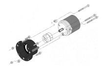
Mounting Examples for Shaft Encoders with Clamping Bracket:
