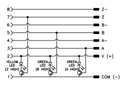
LEDs for indication of channels A, B and Z. Green LEDs indicate channels A and B, while amber is used for the index channel. LEDs can also be used during machine set-up for home position indication, and provide operational status of encoder output
