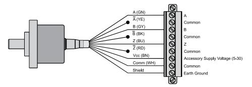
Complements (A not, B not, Z not) should never be tied to common or to each other. The unused wires should be tied back and insulated to prevent them from touching Vcc, common or any other signal wires or driver damage can occur.
