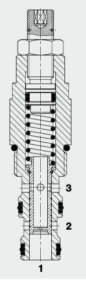
The flow regulator SRP08 is a 3-way spool-type flow regulating valve, with a measuring orifice for controlling flow rate independently of the pressure. The excess flow is made available on the bypass line at port 2. If port 2 is closed the valve acts as a 2-way restrictive flow regulator. If port 3 is closed the valve will stay closed because there is no pressure differential over the piston.
