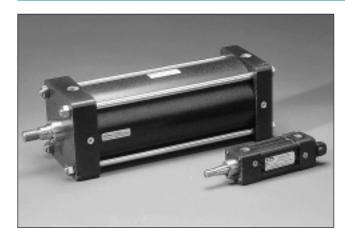
Lightweight pneumatic cylinders by Parker Hannifin's Motion & Control Division were designed for use in harsh applications in the food and beverage industries. Aluminum was used as a replacement for heavier stainless steel in the body, heads, caps, and other components. Prototype units placed in a food plant, however, quickly exhibited severe corrosion due to caustic washdowns. A LECTROFLUOR coating applied to the aluminum parts eliminated any corrosion on their final full-production units.
