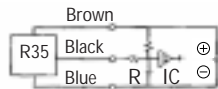
Fig. 6 Protection circuit using current limiting resistor R for capacitive load. Find minimum ohmage from: V/0.15=R(\Omega)
