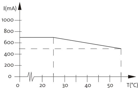
Fig. 10: Derating of the I/O link modules
