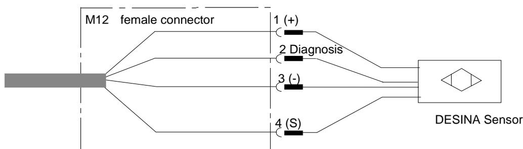
Fig. 11: Connection of Sensors/Actuators with Diagnostic Output
