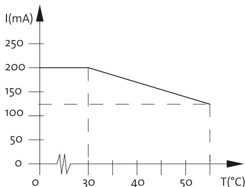
Fig. 9: Derating of the sensor module normal
