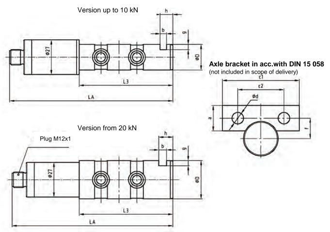
**For two-sided measuring axle mounting the following applies:** Bolt/Hole Mating Tolerances: H9/f9
