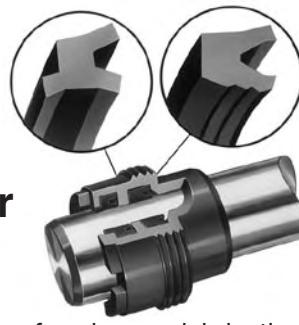
An extra-long inboard bearing surface insures lubrication from within the cylinder. Outboard of the bearing surface are two leakproof seals – The Lipseal and Wiperseal. The serrated Lipseal (primary seal) is completely self-compensating and self-relieving. It adjusts to mechanical deflections or any pressure variation from near-zero to rated operating pressure. The result is positive, no-leak sealing – regardless of conditions.
