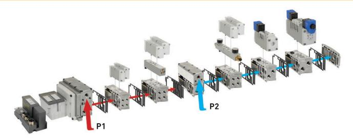
**Pressure Zoning** Multiple Pressure Zones (P1 P2 ... Pn) provide flexibility to meet a variety of applications. Supplying the valves on the manifold with different pressures will allow for variable force output from any attached actuators. In addition, you can control vacuum and remove supply pressure from certain sections while leaving other areas operable. This can be useful in safety applications as well as for maintenance.
