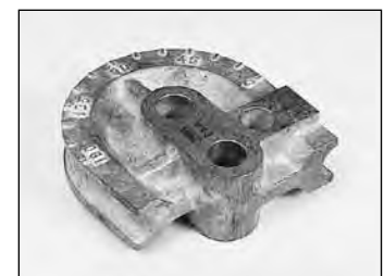
Fig. R27 — Radius Block for use with HB632 Bender
