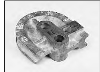
Fig. R28 — Radius Block for use with HB632 Bender
