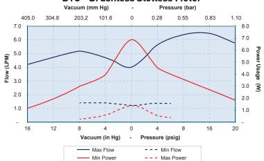
The above graphs represent an example of performance for the pump series handling air at 800 feet (244 m) above sea level at 75 degree F (24 C). Performance will vary depending on barometric pressure and media temperature. A variety of configurations can be accommodated to meet application requirements. Curves are representative of standard pump configurations. Pump configurations could be customized for higher or lower flows depending on specific
