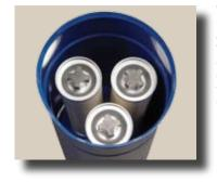
The elements are installed in the housing. They are held in place by a center rod and threaded end cap. This design allows for easy element changeout. The inlet is on the bottom of the housing and the air flows from the inside to the outside. The coalesced liquid collects at the bottom of the internal separator plate and can be easily drained away.
