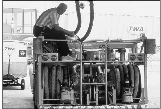
Protecting sensitive meters and small diameter piping from valve closure on fueling trucks
