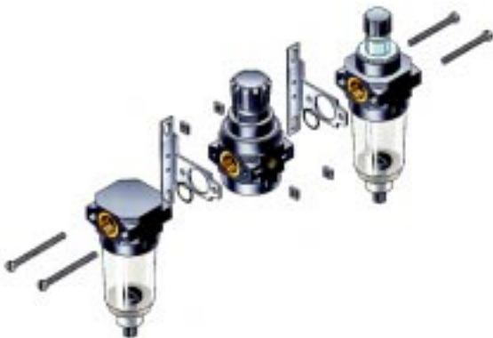
Wall brackets mounted inside an assembly
