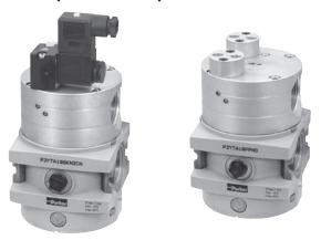
P3Y Series Combined Soft Start / Dump Valves, provide for the safe introduction of pressure to machines or systems. Soft Start / Dump Valves when set, allow the pressure to gradually build to the set point before fully opening to deliver full flow at line pressure.
