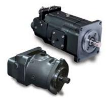
The Gold Cup Hydrostatic Transmission pumps are variable displacement piston pumps of an unparalleled rugged design. Rated to 5000 PSI continuous pressure and continuous duty, the Gold Cup design has the unique feature of an internal servo/replenish and the ability to utilize system over pressure to directly control the stroking chambers. This affords the fastest and most stable control strategy available.
