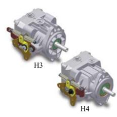
The H3 and H4 Series are manually controlled closed loop axial piston pumps. When paired with Parker's low speed, high torque orbit – type hydraulic motors, they create highly efficient hydrostatic transmissions. These cost effective transmissions are often used as drive systems for the propulsion of off – highway vehicles under 50 horsepower
