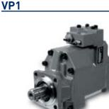
The VP1 is the world's first variable displacement pump for truck applications. It can be close-coupled to a gearbox PTO (power take-off) or to a coupling independent PTO (e.g. an engine PTO) which meets ISO standard 7653-1985.
