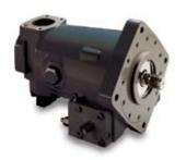
The open-loop Premier Series pumps are variable displacement piston pumps with emphasis on superior design with few maintenance requirements. Low inlet velocity requirements allow the pumps to run faster than competitive models without the added expense of boosting the inlet. Modified pistons that reduce the amount of trapped fluid volume result in improved efficiency.
