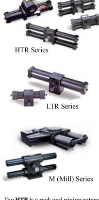
The **HTR** is a rack and pinion rotary actuator in a compact package, providing high power at low rotational speed. The gearing and cylinders are self-contained and protected against contamination, all within a precision machined housing that can be integrated into the end user's product. Heavy duty bearings support large externally applied shaft loads. Standard and custom rotations are available with a variety of options.
