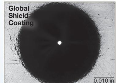
Although a superior rod coating on its own, it *may* also be an **economic alternative to corrosion resistant steels** (i.e. stainless steel) when applied to carbon steel. However, like all coatings, rod end machining would expose the carbon steel substrate, so additional measures
