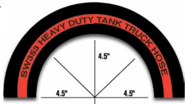
The minimum bend radius is measured to the inside of the curvature.
