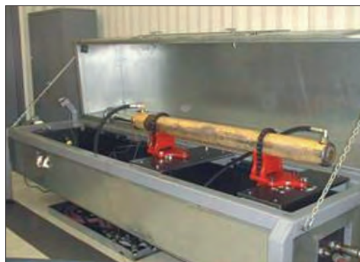
High pressure hydraulic leakage testing
