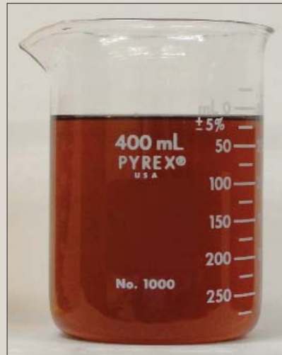
Same samples after 1,300 hours of exposure @ 200°F
