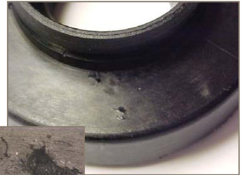
Pitting on filter end-cap
