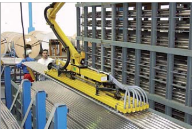
Bellows suction cups FSGB being used for handling pipes
