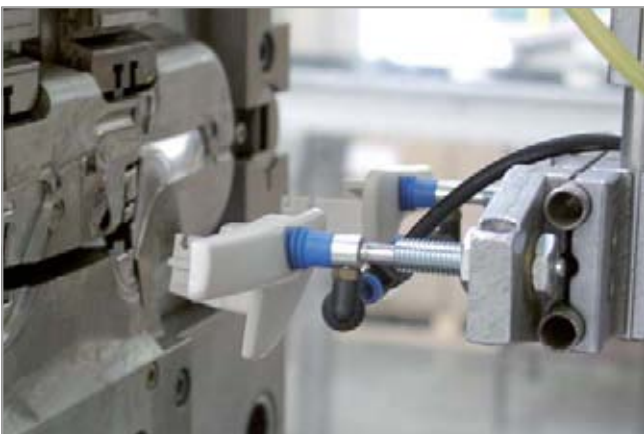
Bellows suction cups FSG being used for handling hot plastic parts
