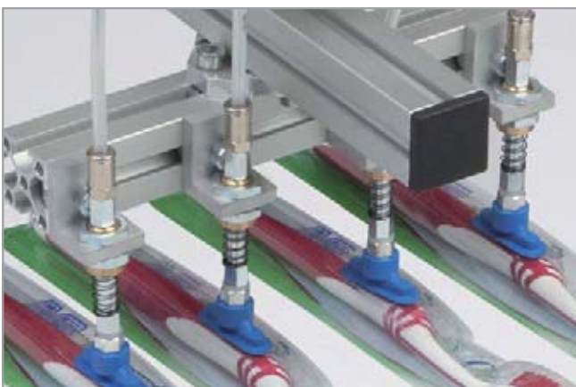
Flat suction cups SGON being used for handling blister packaging
