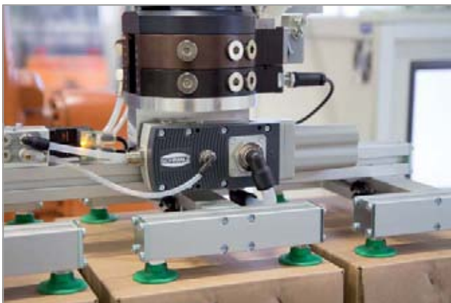
Centralized vacuum generation by means of basic ejectors SBPL
