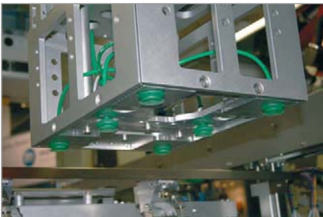
Bellows Suction Cups SPB2 being used in side-loading machines
