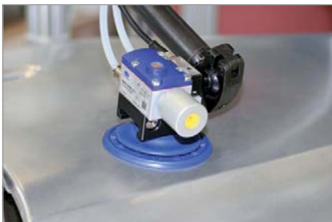
Decentralized vacuum generation with ejector SEAC RP with blow off system right on suction cup
