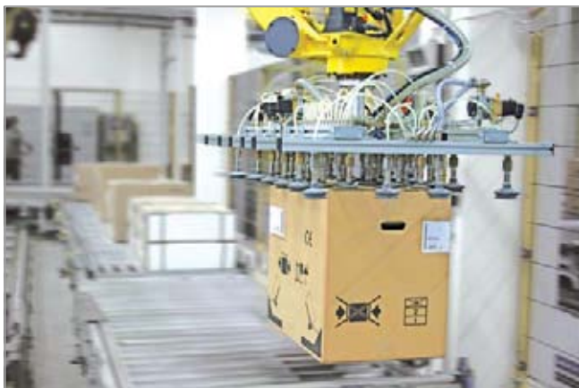
Bellows suction cups FSGA being used for handling cardboard boxes
