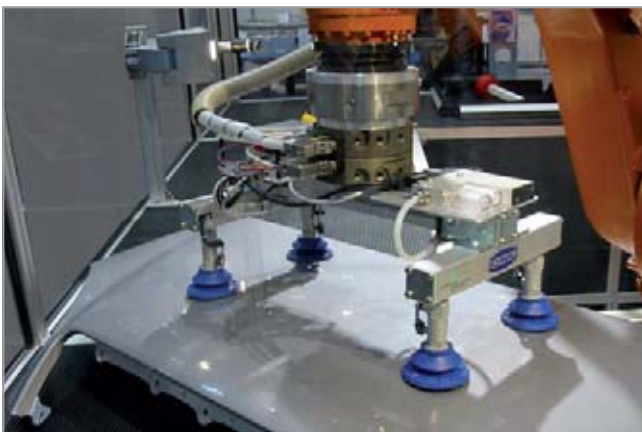
Suction cups with inline valves IV being used for handling car bodywork parts
