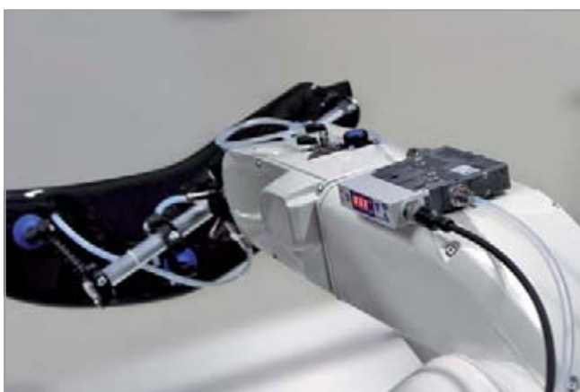
Centralized vacuum generation by means of compact ejector SCPSi
