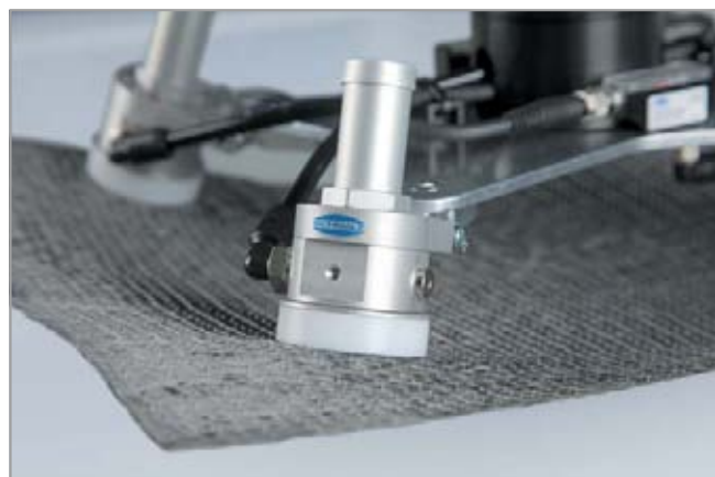
Composite grippers SCG being used for handling composites
