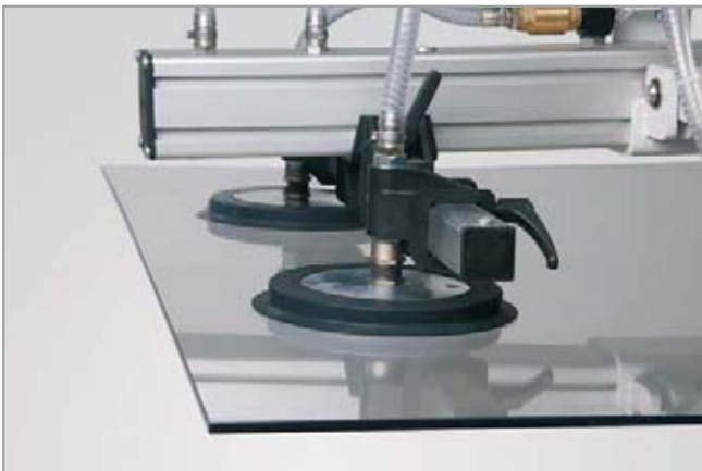
Suction plates SGF being used for handling sensitive glass sheets
