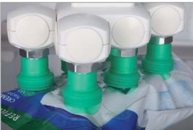
Bellows suction cups SPB4 being used for handling foil-wrapped products
