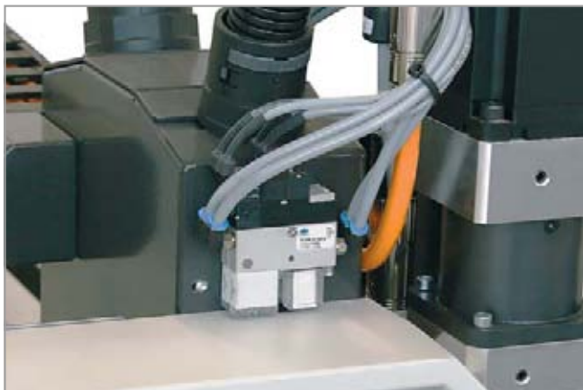
Central vacuum generation by compact ejectors SCPM
