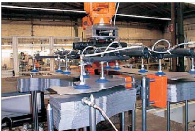
Mounting example spring plungers FSTE-HD
