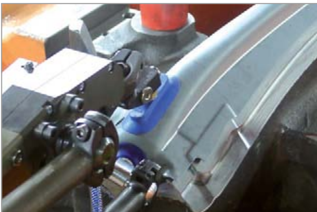
Bell-shaped suction cups SAOG being used for handling very curved sheet metal parts
