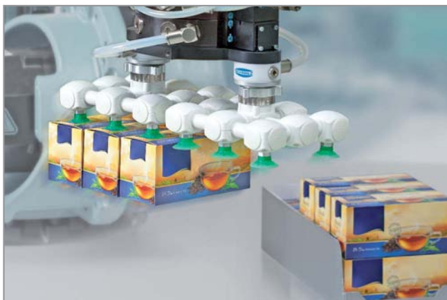
Vacuum end effector with flat suction cups SPF handling boxes of tea
