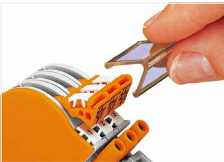
Snapping a transparent locking cover onto 1–8 disconnect links: a) Mechanically lock several links for multi-pole switching applications b) Protect markers
