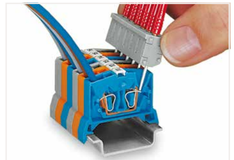
Testing by touch contact to the CAGE CLAMP® spring (limited to 0.5 A and 48 V test voltage) – test pins are not protected against accidental contact.
