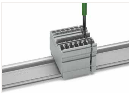
Open the assembly by laterally sliding a block via operating tool (3.5 x 0.5 mm blade).
