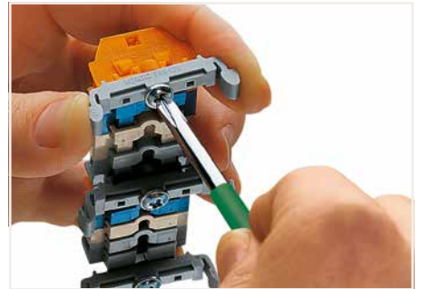
Mounting and securing a terminal strip directly to the plate via screw-type flanges. screwing a mounting foot (209-123) (distance between mounting feet: approx. 20 ... 25 mm)
