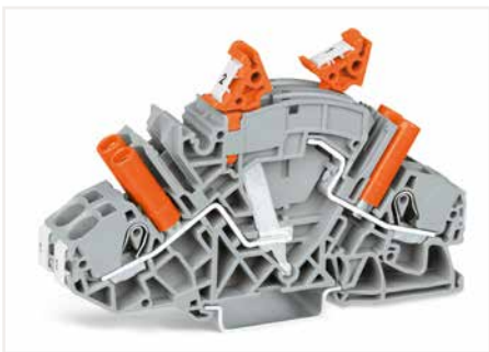
Measurement testing (using both test sockets) Terminal block 1: Disconnect link in operating position I Terminal block 2: Disconnect link in measuring position III
