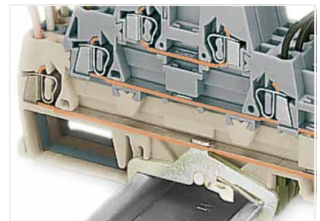
Both ground and shield conductor terminal blocks have a contact foot in the bottom level, automatically establishing direct contact to the DIN-rail or busbar. The flexible marker carrier, which is placed above the wiring level, can be pushed aside during wiring. The carrier has two staggered levels for WMB markers that perfectly align with the terminal block decks. With a terminal block width of just 5 mm, an effective width of just 1.67 mm for terminal blocks of same or different potentials can be realized for conductors ranging 0.08 mm 2 ... 2.5 mm 2 (28 ... 14 AWG).
