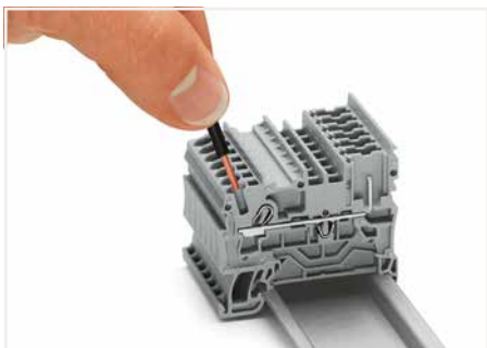
Push-in CAGE CLAMP® enables solid conductors to be connected by simply pushing them into the unit.
