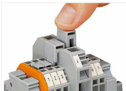
Commoning side-entry rail-mount terminal blocks via step-down jumpers. Push down the step-down jumper until fully inserted.
