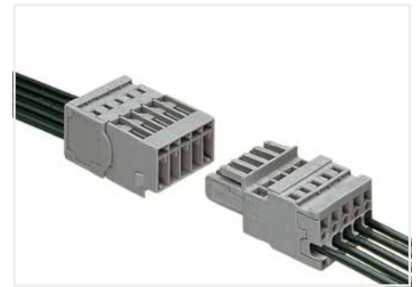
Male connectors with CAGE CLAMP® connection (769-602 to 769-615) Conductor cross section: 4 mm 2 (12 AWG)
