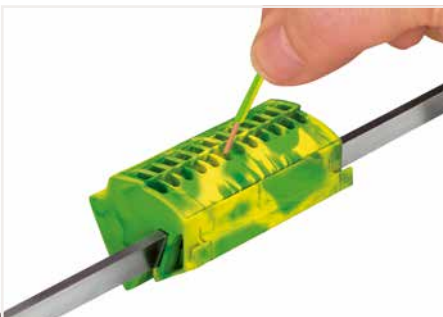
Conductor termination (4 mm 2 /12 AWG): With Push-in CAGE CLAMP®, solid conductors can be terminated by simply pushing them into the 12 x 4 mm 2 busbar terminal block, significantly reducing wiring time.
