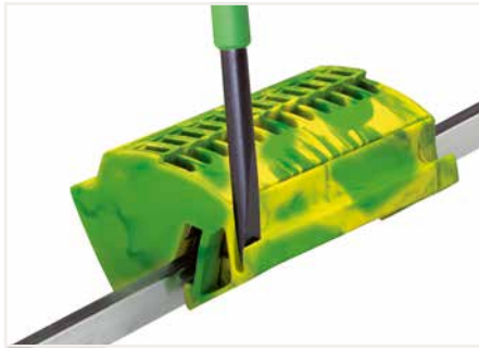
Unlock right and left positions to remove the ground busbar terminal block. Then pull up the block from the busbar.
