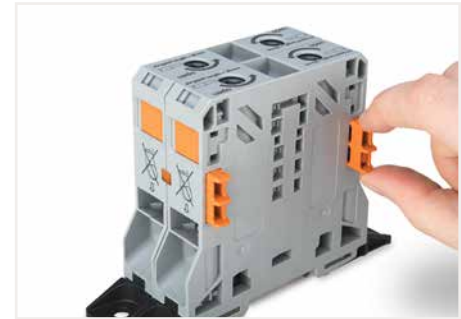
Optionally, insert block-to-block connector (285-448) into housing slot.
