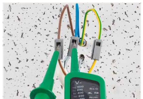
Testing via separate test ports.
