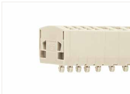
Ex e II terminal strip; with snap-in mounting feet; for 0.6 ... 1.2 mm plate thickness; 3.5 mm mounting hole diameter
