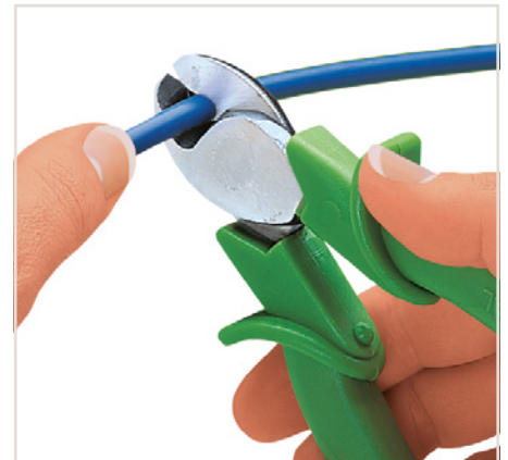
Cutting a cable.
