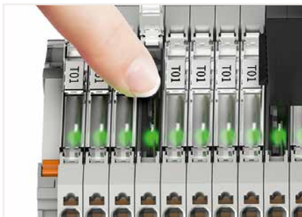
Configuration via push/slide switch
