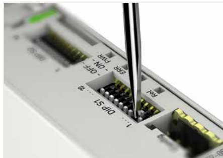
Configuration via DIP switch
