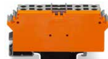
Terminal block for pluggable modules; 8-pole; with 4-conductor terminal blocks; with marker carrier; with orange separator; for 35 x 15 mm and 35 x 7.5 mm DIN-rails; 2.5 mm 2
