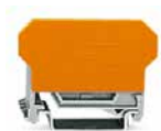
Terminal block for pluggable modules; 4-pole; with 2-conductor terminal blocks; with orange separator; for 35 x 15 mm and 35 x 7.5 mm DIN-rails; 2.5 mm 2
