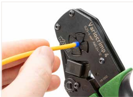
Squeeze handles until ratchet mechanism is released.
