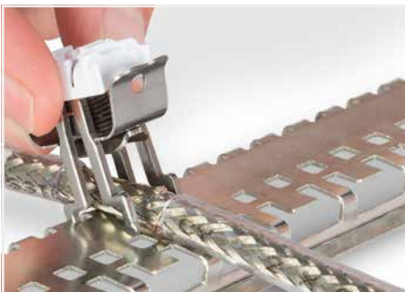
Mounting a clamping saddle on a specialty slotted DIN-rail (790-145). When releasing the saddle, do not place your finger under the clamping spring!
